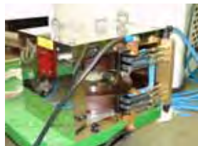
magnet (0.8T), power supply
