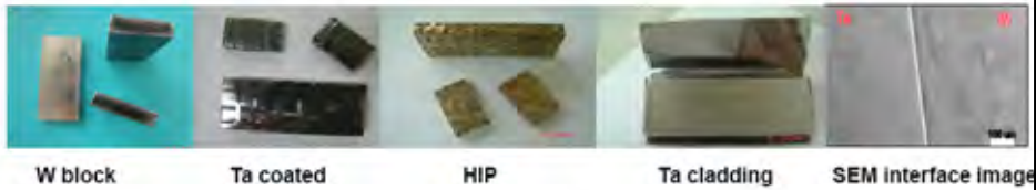
W block Ta coated HIP Ta cladding SEM interface image
