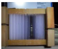
Photograph of the radial collimator made by BATAN
